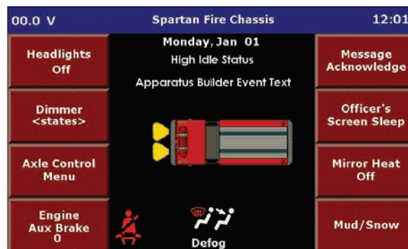
Figure 3-24. Vista IV Standard Controls
