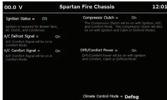
Figure 3-35. HVAC Diagnostics for Single Overhead System
