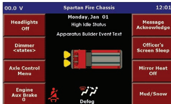
Figure 3-25. Vista IV Interface Features
